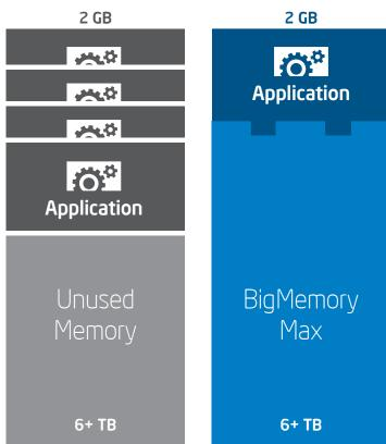
Figure 1. Terracotta BigMemory Max\* creates a data store from unused RAM, which is accessible by applications in microseconds
