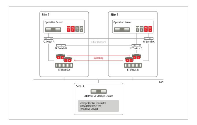
Under normal conditions, VM1 and VM2 at site 1 and VM1 and VM2 at site 2 are connected via Fibre Channel to the respective ETERNUS DX arrays located at the same site – this is called the active (primary) site. All data is synchronously replicated to the standby (secondary) site, while in this example ETERNUS DX 2 is secondary for VM1 and 2 and ETERNUS DX 1 is secondary for VM 3 and 4, respectively.
