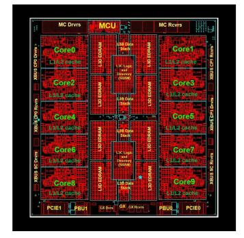
14nm SOI Technology 17 layers of metal 6.1 Billion Transistors Chip Area 26.5 x 27.8 mm
