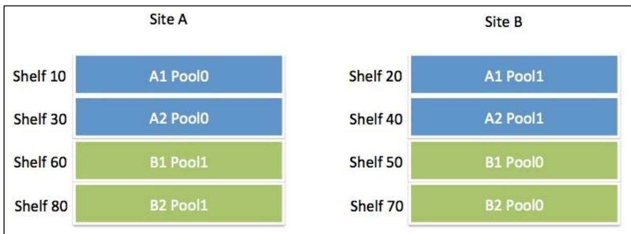
If SSDs are included in FibreBridge-attached stacks, see the [Interoperability Matrix Tool](#) for the supported maximum stack depths. Up to 48 SSDs can be present in any single disk stack, and the SSDs can be distributed across any of the shelves. However, NetApp recommends that you not mix SSDs and HDDs in the same shelf, and that you instead configure SSD-only shelves.
