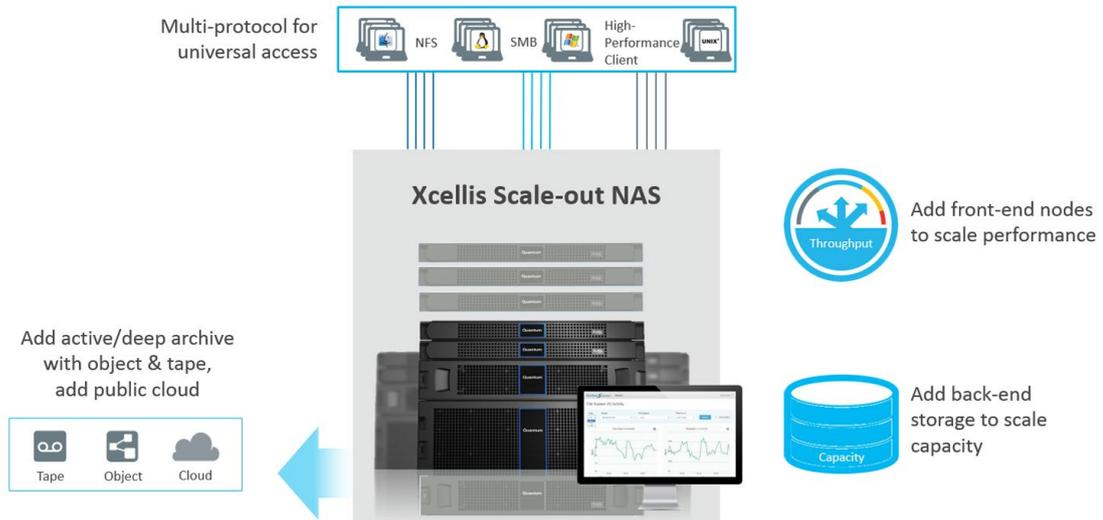
Today an Xcellis Scale-out NAS can manage up to 10 billion files and has a theoretical peak capacity of 512 LUNs and 18 exabytes.
