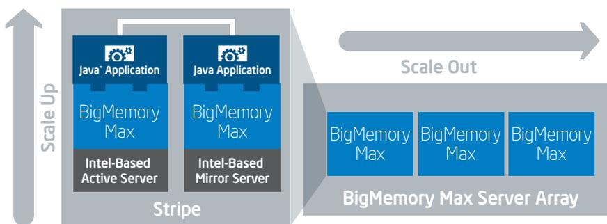
**Figure 2.** Terracotta BigMemory Max\* can pool RAM from multiple servers in an array configuration, and provides high availability and resiliency by mirroring the data across two or more servers in an array configuration
